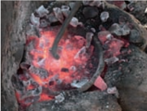
Air from the bellows' nozzle raises the temperature of the charcoal over the small area of the crucible.
